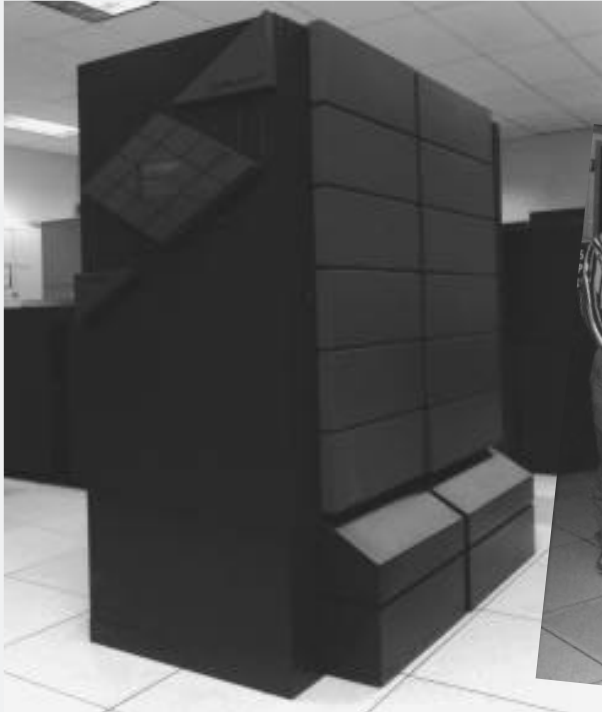
At left: The Cray T3D was delivered to our Advanced Computing Laboratory in June 1994. It is a 128-processor machine that will be used primarily for collaborative research with industry. Below: Scientists and engineers from Cray Research, Inc. and Los Alamos at a dedication of the new machine.
